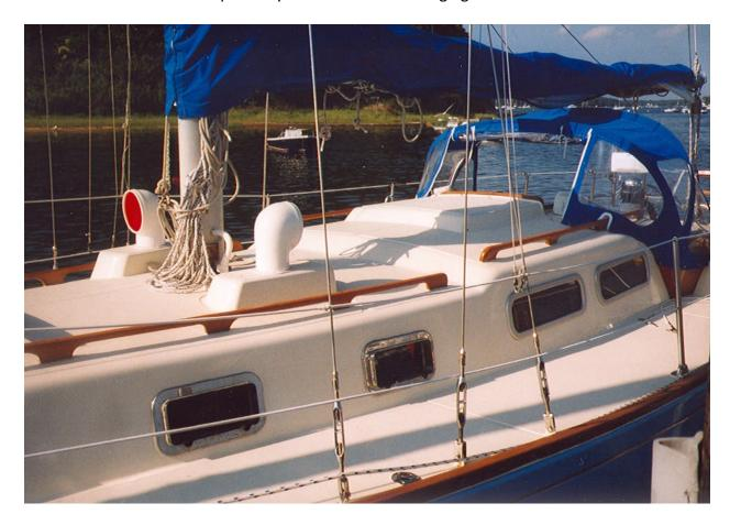
I fabricated a couple of bronze pieces to cut into the toe-rail to facilitate drainage through the toe rail and a couple of bow chocks which are also cut into the Toe-Rail.
