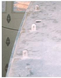
Toe-rail screws and the deck hull screws. They are evenly spaced. Most came apart without holding the top slot in the screw.
