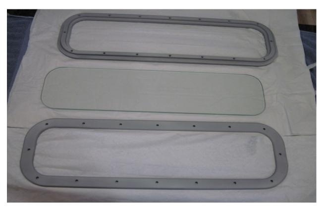
The blind holes were drilled in the exterior frame and tapped for ¼ -20 Stainless Helicoids to help prevent electrolysis between the dissimilar metals (Stainless Crews and aluminum frames)
