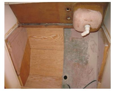
located too close to the new holding tank). The entire area was cleaned and painted with Interlux barrier coat (2000/2001)
