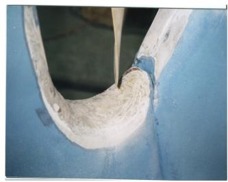
Picture of complete aperture ground to increase opening to fit 14 inch Prop. Completed aperture opening with new Prop
